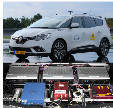
Fig. 4: TNO Renault Grand Scenic (2018) testing platform.
